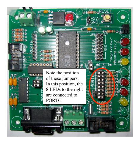
The configuration of the development board is such that +5 volts is connected through a resistor to one leg of each LED, and the ground for each LED is attached to a pin on PORTC. This means that when a pin on PORTC is set high (+5 volts), there is no current flowing through the LED and the LED is off. When a pin on PORTC is set low (ground), current flows through the LED, and the led is on. So, for this setup, turning a pin off, turns the LED on.
