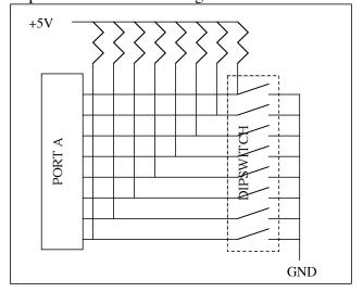
This dipswitch circuit works similar to the LEDs on the development board. When a dipswitch is closed, the corresponding pin on PORTA is brought low. When a dipswitch is open, the corresponding pin on PORTA is brought high. If we write a program that maps the value from PORTA to PORTC, we will have a circuit where closing a switch attached to PORTA lights up the corresponding LED attached to PORTC.
